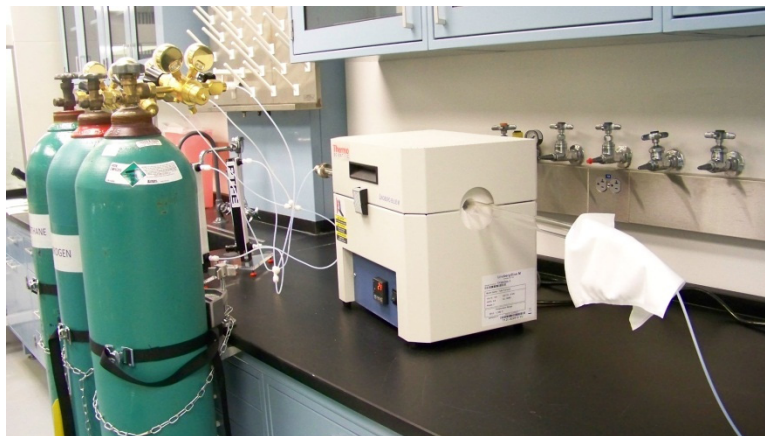
Figure B-1 Home-made chemical vapor deposition furnace for the growth of graphene and pyrolytic carbon.
